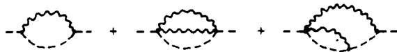
Figure 2. Absorptive parts of \Sigma in the integral equation for the meson propagator.
